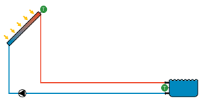
Direct flow-through, intelligent pump control
