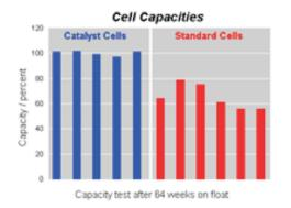
Maintain cell capacity - Many VRLA cells in service are failing capacity tests because their negative plates are depolarized. In fact significant capacity increases have been seen on some cells just by installing a catalyst.
